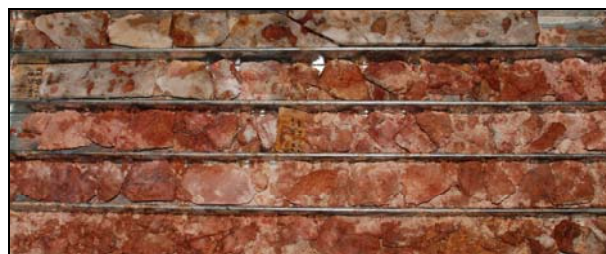
Fig. 5. Intensely altered core of the drill hole PDIC-04-01
