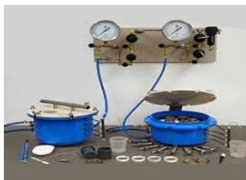
Figure 2. Preparing soil/substrate and placing samples on Bar extractor and Porous plate extractor
